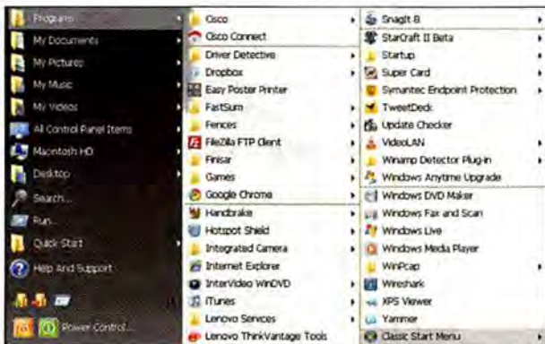
THE $20 CLASSIC Start Menu app transforms Windows 7's scrolling All Programs list into a fly-out list similar to that of Windows XP.
