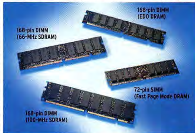
FIGURE 1: DIFFERENT MEMORY MODULES look very similar and bear cryptic markings. Check the original packaging to confirm what yours is.
