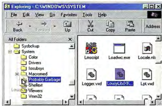
FIGURE 1: MOVE SYSTEM FILES you think you don't want (instead of deleting them), so they're easy to replace if needed.
