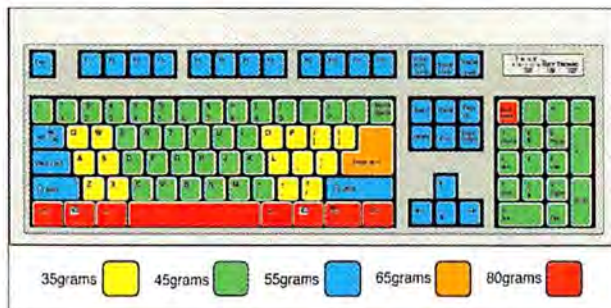
KEY TRONIC'S ERGOFORCE keyboard varies the amount of pressure required for different keys, making typing more comfortable.
