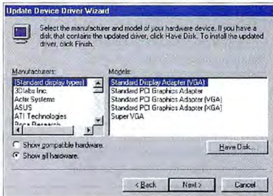
FIGURE 1: INSTALL WINDOWS' VGA DRIVER before you remove your old graphics card and install a new one.
