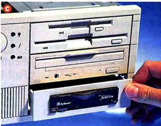
**4 Hook up an external SCSI drive.** If your PC doesn't have an add-in SCSI card, you'll need to install one (A). Shut down your PC, remove the cover, and follow the directions that came with the card. (For more on installing SCSI cards, see the June 1997 *Upgrade Guide*.)
