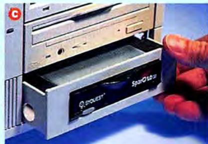
**3 Hook up an internal SCSI drive.** If your PC doesn't have a SCSI card, install one. Shut down your PC, remove the cover, and follow the directions that came with the card. (For more on installing SCSI cards, see the June 1997 *Upgrade Guide*.)
