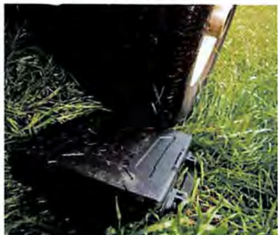
The only damage sustained by the Panasonic CF-25 after we drove an Isuzu Trooper over it was a muddy tire track.
