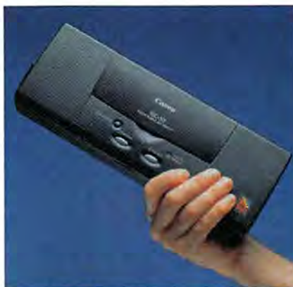
PETITE AND PORTABLE: The BJC-50 can print about 100 pages with its built-in battery.
