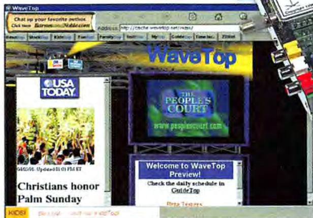
WITH A TV TUNER CARD and WaveTop software, you can have Web pages delivered to your PC via a little-used portion of the TV signal.
