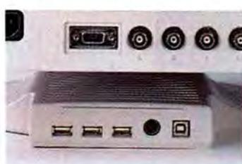
SAMSUNG'S 700Up tucks a three-port, self-powered USB hub in its base. Better yet, the monitor's innovative control software actually makes it fun to tweak your display settings.
