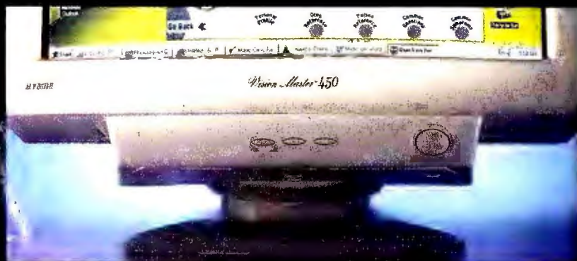
IYAMA USES FEWER BUTTONS: You access most of the individual controls by using the on-screen display's menu system.
