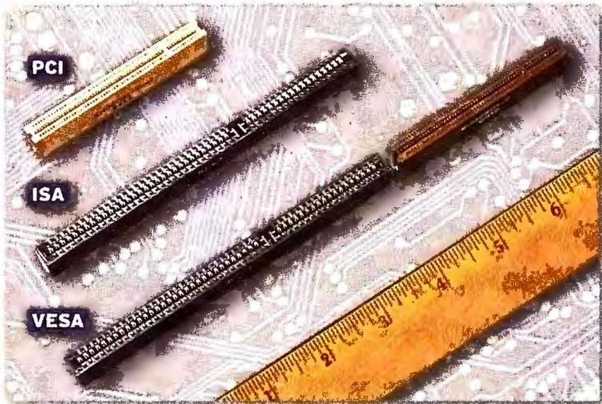
**1 Make sure you've got a PCI slot.** Before purchasing your new graphics board, make sure that your computer can handle the latest cards. Most PCs made during the last three years have PCI slots, but examine yours. Check your manual, or open the PC case and find the existing graphics card (attached to the monitor). If necessary, remove the card and look at its slot.
