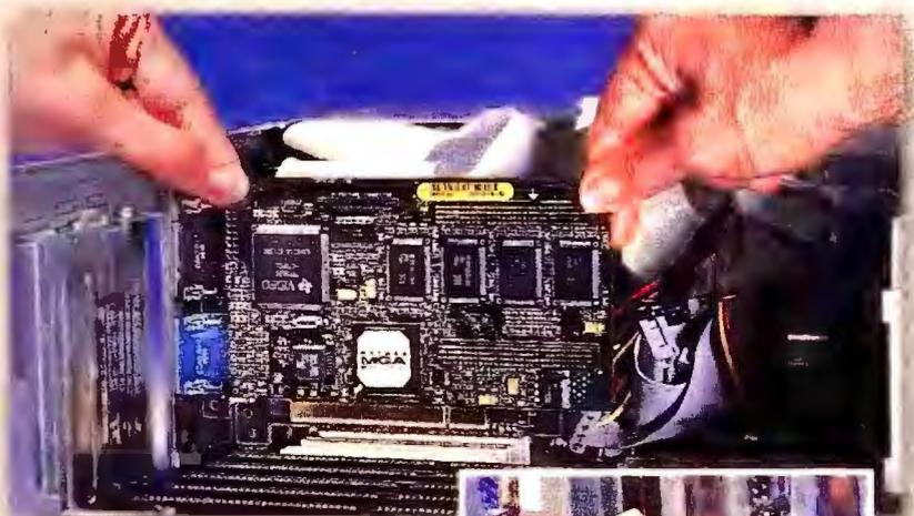
**4 Plug in the card.** Unplug your monitor's graphics connector, take off your PC's case, remove the screw holding your existing graphics card, ground yourself by touching the PC case, and remove the old card.
