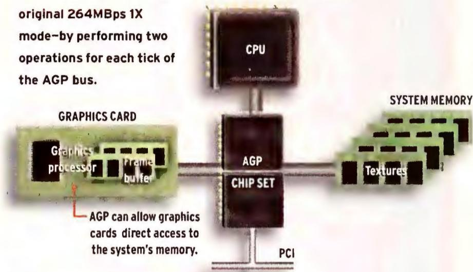
**How AGP works** AGP promotes your graphics card in the PC's data food chain. It creates a new connection between the graphics card and system memory, so graphics data no longer travels on the busy PCI bus. The 66-MHz bus—twice the speed of the PCI's—provides fast access to RAM for displaying realistic 3D graphics.
