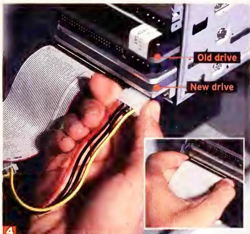
**4** Connect data and power cables. Mount your new drive. You may need an adapter kit and a pair of drive rails to allow a 3.5-inch hard drive to fit into a 5.25-inch bay.
