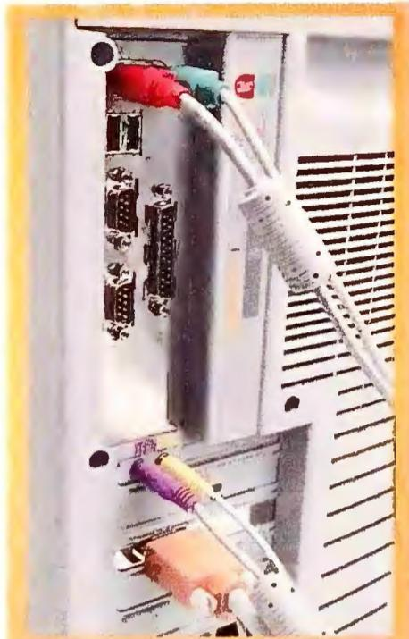
**COLOR ME CABLES:** With color-coding, PCs are easier to assemble.
