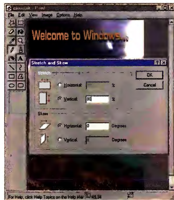
FIGURE 2: SQUEEZE A 256-COLOR BIT MAP into 320 by 400 pixels and use it to replace the Windows 95 start-up logo.
