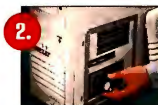
2. Remove the right-side quick access panel to install CPU, cache and RAM.
