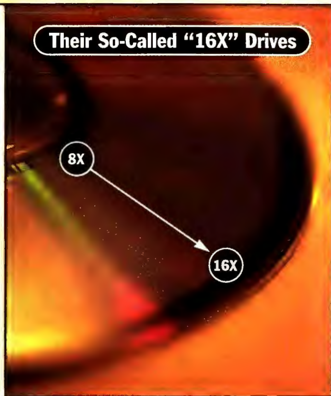
Their 16X CAV Drives starts reading at 8X, and only reads at 16X at the end of the disc, a drive rating of 11.5X*
