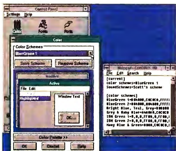
FIGURE 1: EXPORT COLORS IN WINDOWS 3.x by copying the appropriate lines from one system's control.ini file to another's. When you open the Control Panel that contains the copied colors, choose from the schemes you transferred.
