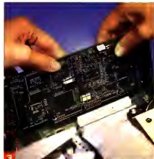
**In with the new.** Find a free slot (most sound boards use standard ISA slots). If you're connecting a CD-ROM drive to the sound board, use the slot closest to the drive. Carefully insert the board in the slot, and tighten the screw that holds the board in.
