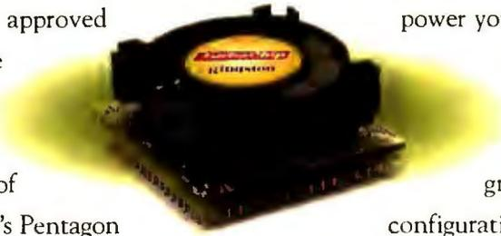
performance improvement.\*" The TurboChip's 5x86 clock-quadrupled technology helps your system run up to three times faster with all the power you need to run today's demanding software. Designed with AMD's Am 5x86-P75 CPU, it upgrades most IBM-compatible desktop systems. And since the TurboChip is a chip-for-chip replacement upgrade, it's easy to install. Plus, it preserves your system configuration. Call today to find out why the military says,
