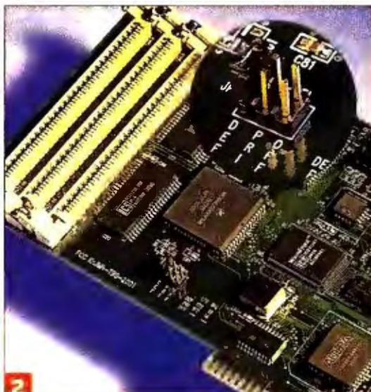
**Check the jumpers.** Some sound boards still make you set jumpers manually before connecting CD-ROM drives—check your manual for details. If your CD-ROM drive is connected elsewhere or you don't have one, set the IDE jumper to Off.
