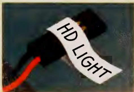
FIGURE 1: LABEL THE LITTLE WIRES from the hard disk light, reset button, and other components so that they're easier to attach to the new board.
