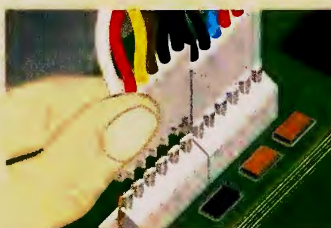
FIGURE 2: DON'T YANK POWER CONNECTORS upward; to remove them, snap them forward. They are keyed so you can't plug them in the wrong way.
