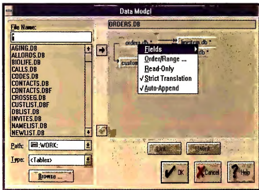
YOU'LL FIND PARADOX'S AUTO-APPEND FEATURE, which lets you add new records easily, in a properties menu of the Data Model dialog box.
