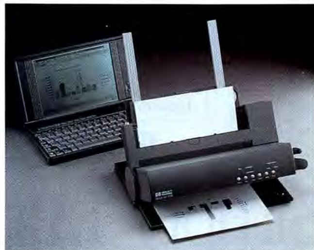
PRINTER COMPANION: HP'S DESKJET 310 weighs 7 pounds and provides 300-dpi color printing on the road.
