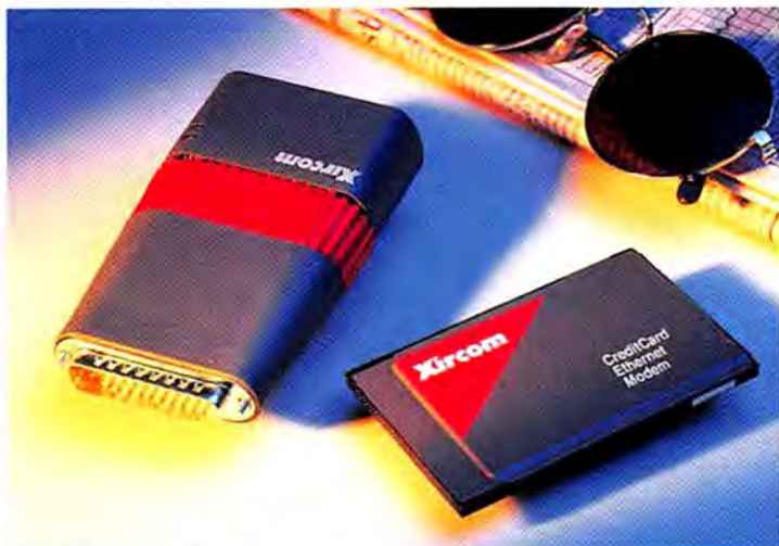
ALL-IN-ONE MODEM AND LAN ADAPTER: Xircom's new Ethernet+Modems combine a 14.4-kbps modem and a 10-mbps LAN adapter into one small package.
