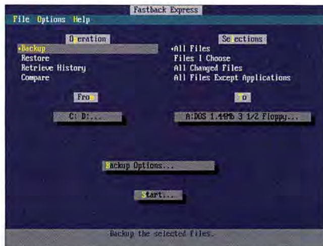
EASY BUT LIMITED BACKUPS: Novell DOS 7 comes with Fastback Express, a backup utility from the now defunct Fifth Generation Systems. The user interface is nice, but it can't back up to tape drives.
