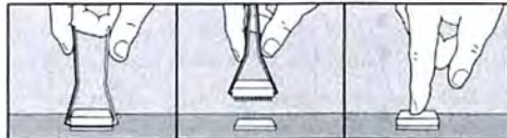
Here's how to get an instant 486. Just use the chip removal tool provided to pull out your 386DX chip (16, 20, and 25 MHz versions), and plug our Cyrrix Upgrade Microprocessor into the empty socket. Installing the SX version is even easier. It just clips on over the existing chip.
