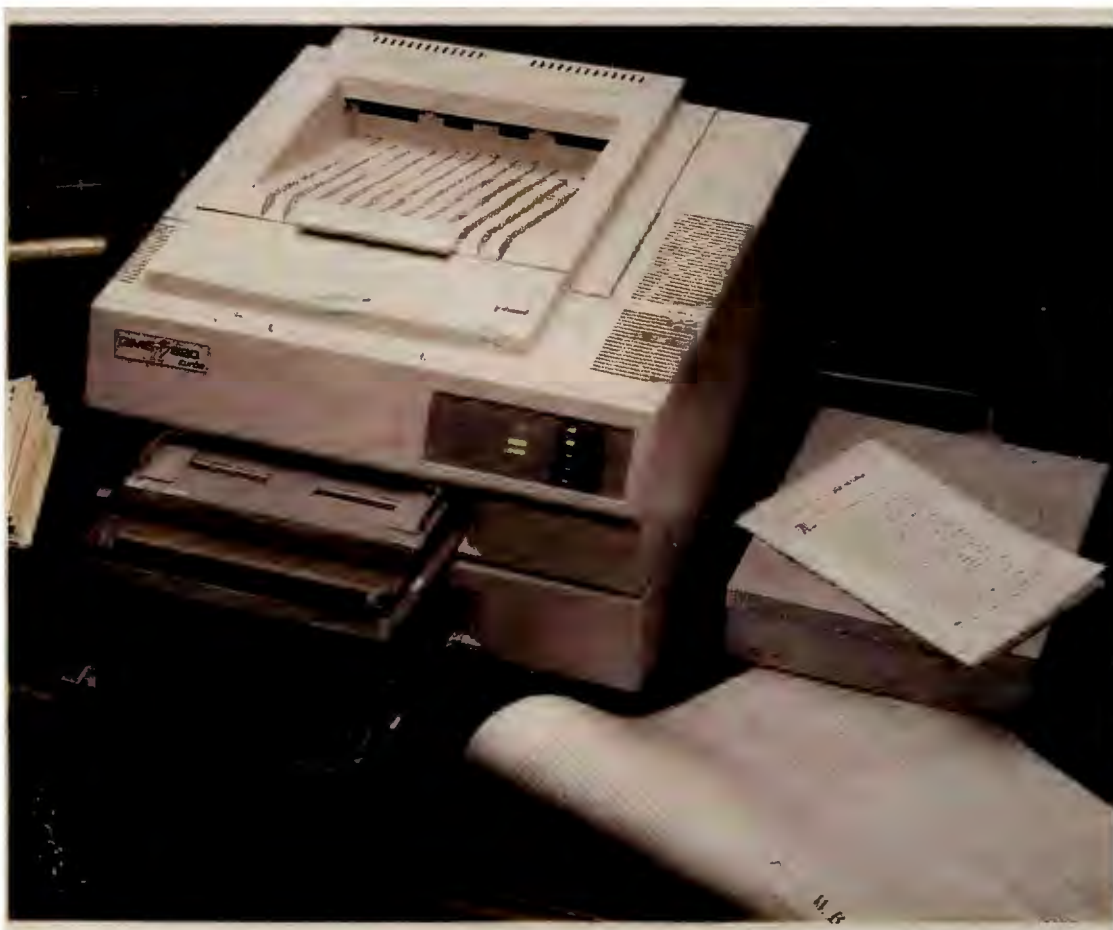
The QMS-PS 820 Turbo has solid network credentials, including multiple paper trays and an interface for hooking up a SCSI hard disk (such as the Apple drive shown here).
