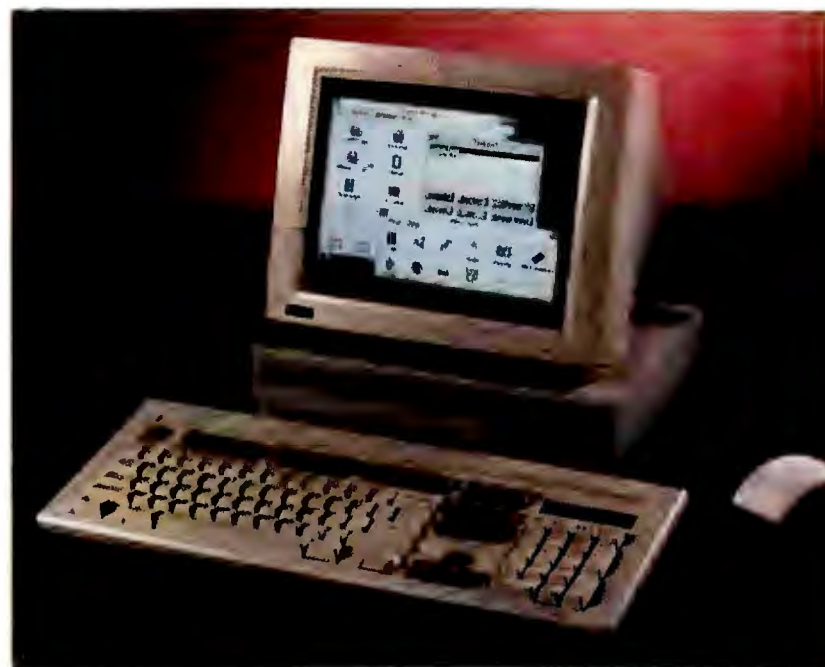
A high degree of integration on the motherboard makes the Infinity Desktop as much as 12 square inches smaller than other 386SX systems.
