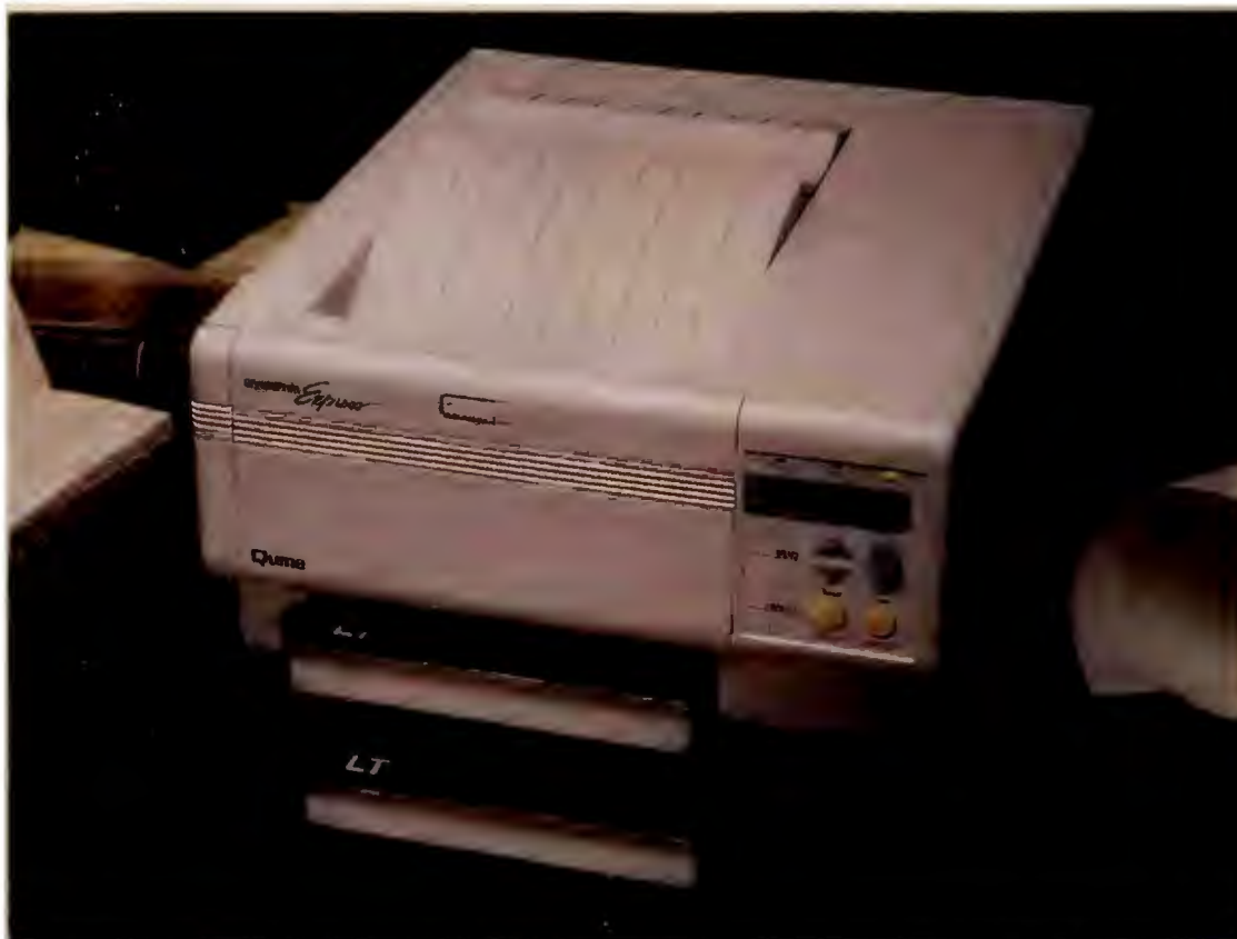
The Qume CrystalPrint Express produces fast, high-resolution output, but don't bother looking for a hard disk interface or font cartridge slots—there aren't any.
