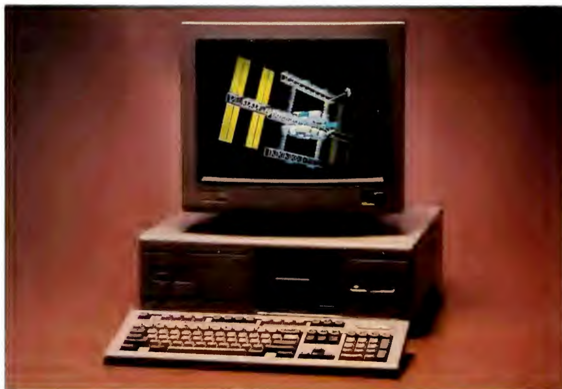
The Deskpro 386/33 is 32 percent faster than 25-MHz models, has two more expansion slots, and holds two 650MB hard drives.
