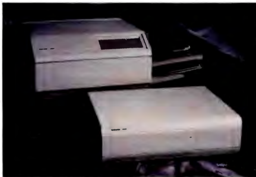
A PostScript-compatible printer, the Tektronix Phaser CP uses a thermal wax-transfer process to bring you 300-dpi color output.
