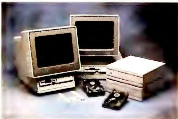
IBM® PS/2 Models 25, 30 and 30-286 Solutions: (INTERNAL) 20, 30 and 40 MB; 40-24 ms. (EXTERNAL) PC Stack: 30, 45 and 80 MB; 40-28 ms.
