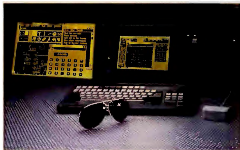
The 20-pound Dolch P.A.C. 386/25 lets you take 25-MHz, zero-wait-state performance on the road with the help of a 64K disk cache. The unit is backed by a 19ms 40MB hard drive with its own proprietary cache scheme for optimum speed.
