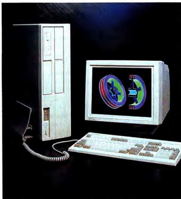
Zenith's Z-386/25 offers up to 32MB of 32-bit memory, 16K of 25ns cache, and a choice of fast ESDI drives with 1:1 interleave controllers for your biggest computing jobs.
