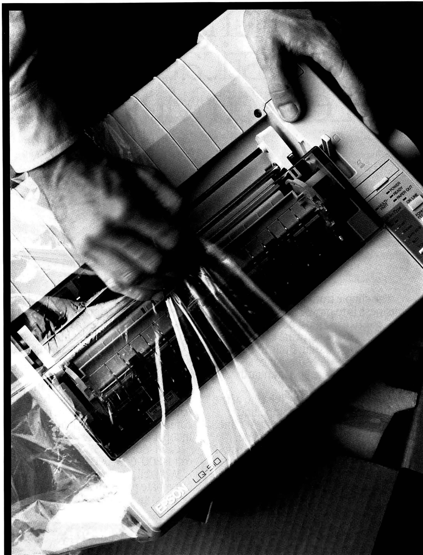
Epson LQ-510. Narrow-carriage 24-pin printer, 180 CPS/draft, 60 CPS/letter quality, built-in push tractor, auto single sheet load, bi-directional printing for both text and graphics, four resident fonts. Epson LX-810. Narrow-carriage, 9-pin printer, 200 CPS/SuperDraft, 180 CPS/draft, 30 CPS/near-letter-quality, built-in push tractor. One year limited warranty on both printers. Epson is a registered trademark of Seiko Epson Corporation. SmartPark is a trademark of Epson America, Inc., 2780 Lomita Blvd., Torrance, CA 90505. (800) 922-8911.
