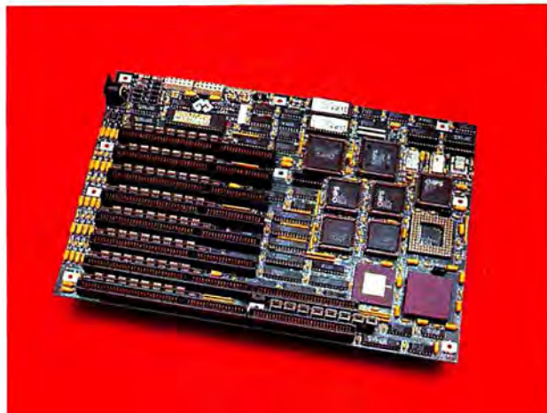
The MicroFrame 386CT motherboard turns an AT into a zero-wait-state 386 with a choice of processor speed, memory, and expansion options.
