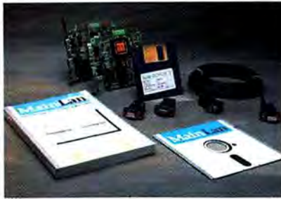
The MainLan Starter Pack—everything you need to connect two computers, including two network boards, software, documentation, and one 16.5' shielded cable with terminating plugs. The Extension Pack contains the network board, and one cable and plug set.
