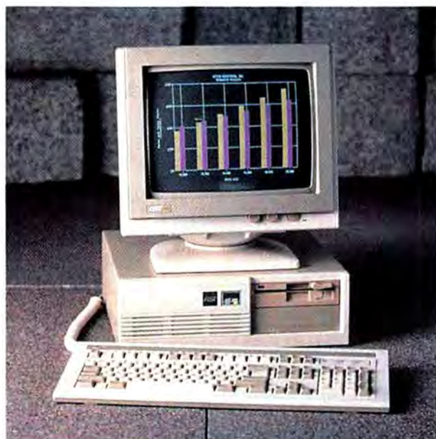
The 8-MHz, zero-wait-state AST Bravo/286 employs AST's custom ASIC, surface-mount, and VLSI technologies to provide maximum expandability in a small footprint. It still offers one 8-bit and three 8/16-bit expansion slots and holds two half-height storage devices.
