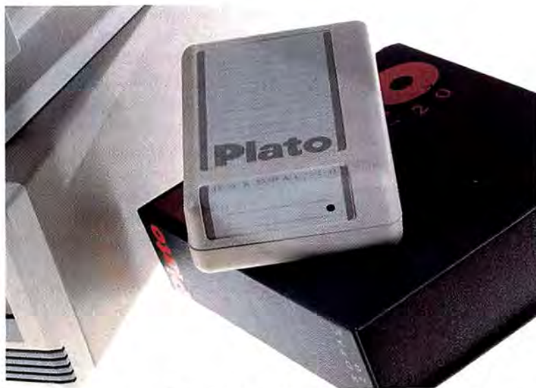
Hard to install, easy to use: The Hardpac 20 must be set up on an XT, but it's perfect for quick backups and cheaply sharing hard disk storage.
