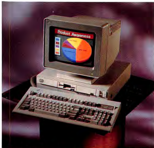
The IBM Model 30 286 is the first PS/2 to revert to the AT bus. VGA is built in, but the only hard disk IBM offers is a low-capacity 20MB unit.
