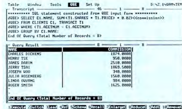
Quadbase Systems' dQUERY 2.1 Query by Example interface lets you formulate queries by making entries in forms on screen. A limited SQL interface is also included.
