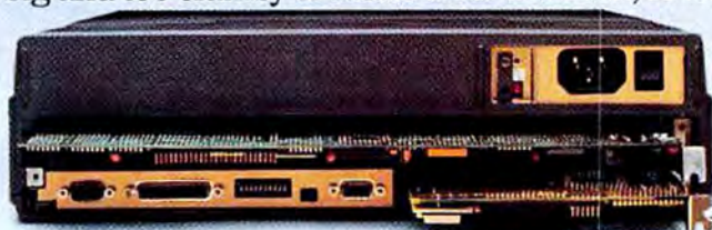
Two IBM-compatible internal expansion slots let you expand the T3200's capabilities quickly and easily.
