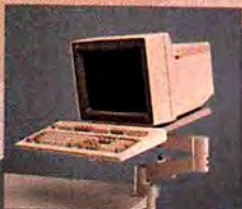
Shown with keyboard holder option. Arm holds 60 lbs. Tilts \pm 10^\circ . Rotates 360^\circ . Adjusts 7 3/4" to 12" above desktop.
