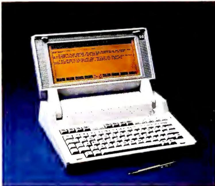
Hewlett-Packard's Portable Vectra CS can be used as a desktop at the office with the addition of a full-size monitor.
