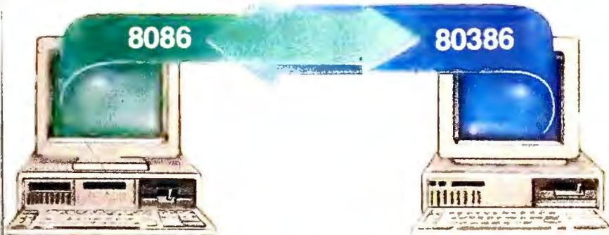
80386-based PCs & PS/2s are dual-personality computers. To run DOS programs, they act as PCs with a 640K memory limit. But to take advantage of their minicomputer capacity, they operate in true 80386 mode which lets them address up to four gigabytes of memory. PC-MOS enables the 80386-host and its workstations to independently switch between these modes—making DOS compatibility and 80386 power simultaneously possible.
