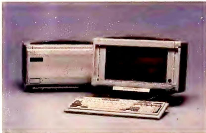
Compaq's 20-pound Portable 386 has the same design and 10-inch gas plasma display as its Portable III, but with a 20-MHz CPU.
