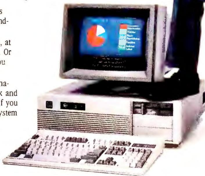
**TRANS/PRO 9™** Superb Intel 80386 CPU ticking at 16 MHz; 1 MB of RAM on the motherboard; floppy and hard disk controllers; 1.2 MB floppy disk; monochrome or color graphics card; integral 9-inch monochrome monitor; eight, full-length expansion slots; and snap-on, 83-key keyboard with soft-touch keys.
