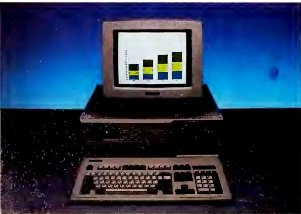
The Acer 1100 is the only one of the three machines reviewed to offer 80387 coprocessor support. At \$4895 for a unit with a 40MB hard disk and an EGA display, it's also the cheapest.
