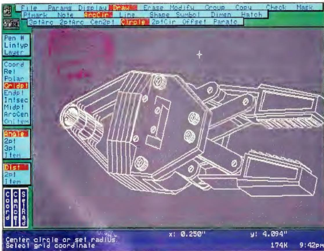
A typical *Drafix 1 Plus* screen showing a sample drawing of a robotic gripper. The three vertical stripes in the lower left corner represent the three mouse buttons, each labeled to show the current effect if clicked.
