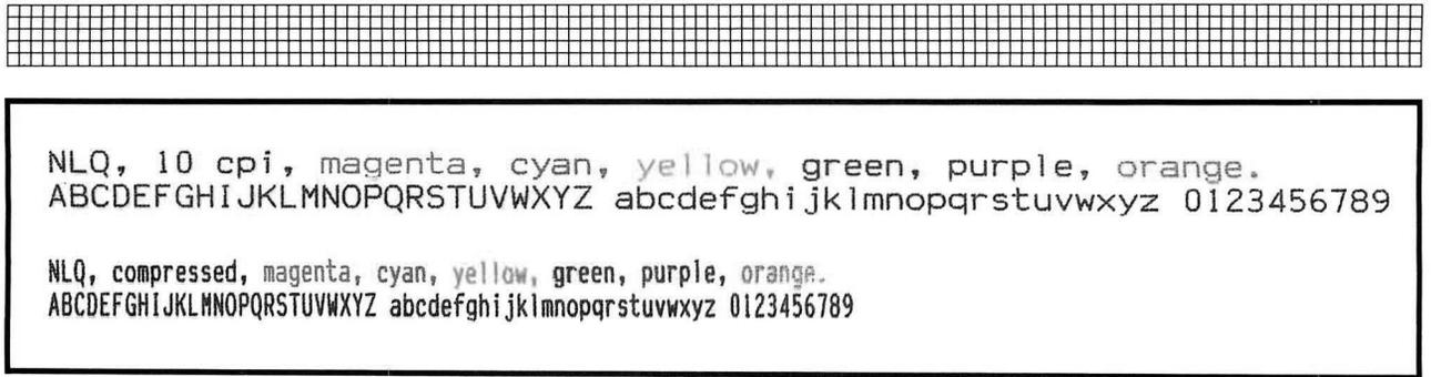
Figure 1: The NLQ text produced by Texas Instruments' Model 857 Color Printer is fairly sharp, but the descenders on some letters are sometimes indistinct.
