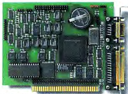
Overboard. ™ EGA or mono/color graphics, serial and parallel ports, plus clock on a short card.
