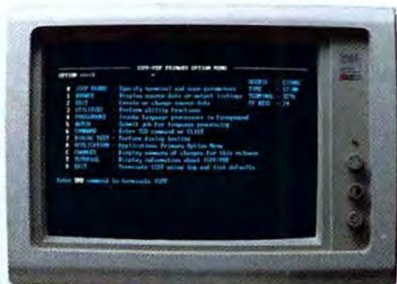
PCOX/STANDARD links a PC direct to the mainframe. PCOX/PLUS (not shown) can "window" a PC session, host session and two notepads on the same screen.
