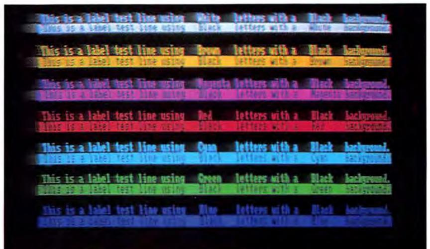
Figure 6: A series of colored labels on an RGB monitor
