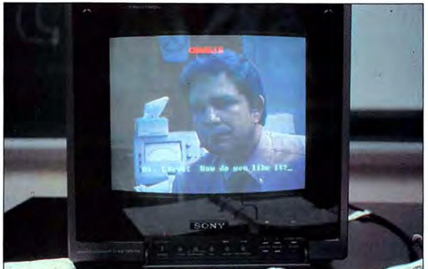
Figure 5: A composite video and RGB overlay. The RGB signal is from an IBM PC; the composite video is from a JVC KY 19000 CH camera.
