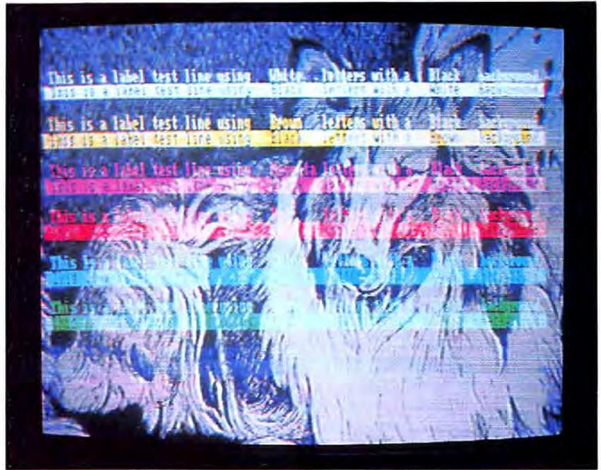
Figure 9: A composite video picture of a pen and ink drawing with an overlay of colored labels
