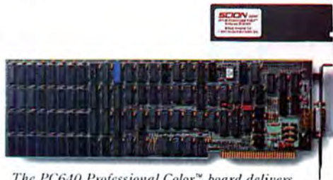
The PC640 Professional Color™ board delivers superior resolution at 640 x 480, and the simultaneous use of 16 out of 4096 colors.
